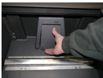
2. Removal is a simple process of pushing the rear of the plate up which lifts the rear pegs clear of the housing
