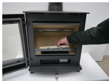
1. Remove the front base brick part
