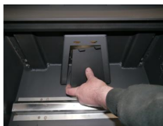
3. Twist the steel baffle as the rear pegs disengage from the housing to remove
