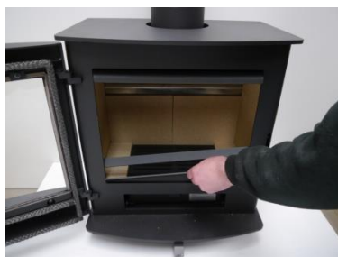
2. Gently lift the front fence up and out of the stove followed by the grate and remaining base bricks
