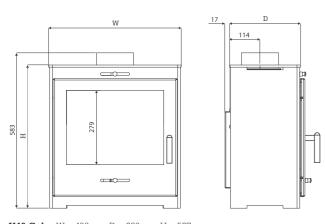
$\begin{array}{l} \textbf{X40 Cube} \ W = 496mm \ D = 280mm \ H = 537 \\ \textbf{X60 Cube} \ W = 496mm \ D = 396mm \ H = 537 \\ \textbf{X40 Cast Iron door} \ W = 545mm \ D = 308mm \ H = 605 \ \text{All Measurements in mm} \end{array}$
