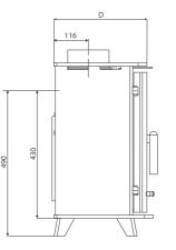
$\textbf{40FS} \; D = 304mm \;\; \textbf{50FS} \; D = 348mm \;\; \text{All Measurements in } mm$
