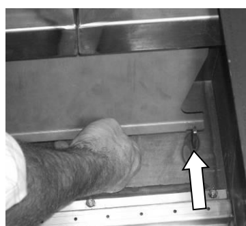
1. Lift the rear of the steel baffle up to clear the rear locating pegs and ease it backwards
