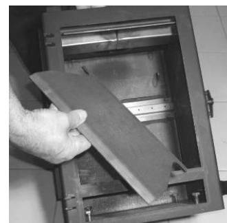
3. The baffle can now be lifted off the rear pegs and tilted out of the stove. Assembly is the reverse.
