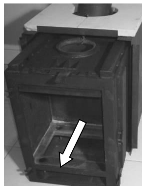
Fig E Slide stove out of outer convection casing
