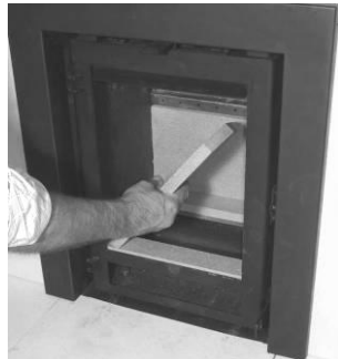
2. Carefully remove the left hand fire brick
