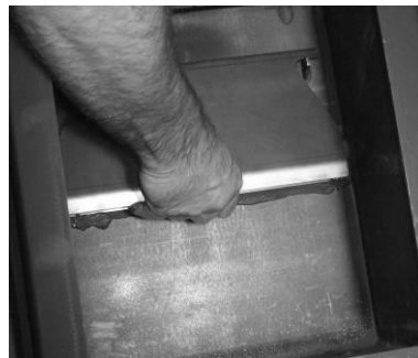
2. As you move the baffle back it will disengage from the front support slot allowing it to be rotated down on the rear pegs
