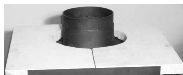
Skamolex blue (calcium silicate) insulation material
