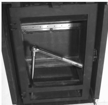
Fig D Undo the adjustable feet with a 17mm socket
