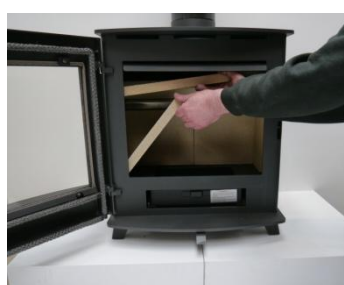
3. Ease the left hand side brick away whilst supporting the front baffle section with your other hand. Carefully manoeuvre both baffle brick sections out of the stove
