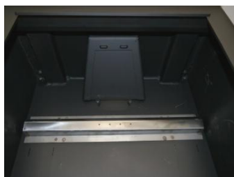
1. The upper steel baffle sits in a bolt-up housing at the top of the inside of the stove
