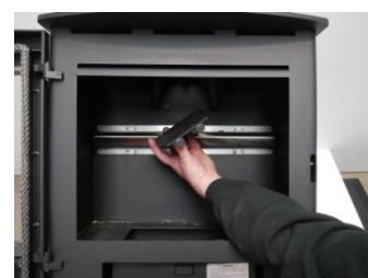
4. Removal of the baffle gives immediate access to the flue for sweeping and maintenance
