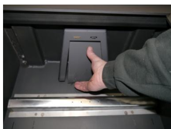
2. Removal is a simple process of pushing the rear of the plate up which lifts the rear pegs clear of the housing
