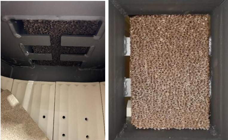
Catalytic converter mounting above the ball catch behind the smoke deflector for M, Maestro, QM40 ecoline
